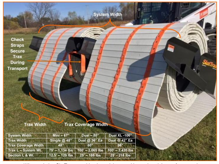
When ordering SlatTrax, consider the weight capacities and track base of your equipment. Additional sections of Trax can be added to the system as required.
