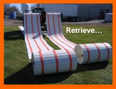
Connect Trax to Spool Harness - Back up and Begin Roll up of Trax onto Spools
