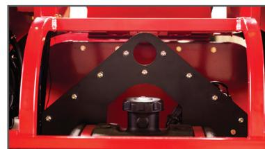
A single point lifting hook can be found under the seat.
