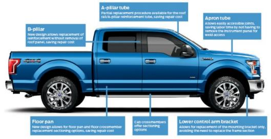
The F-150 was designed and built with modular construction methods to reduce repair costs
