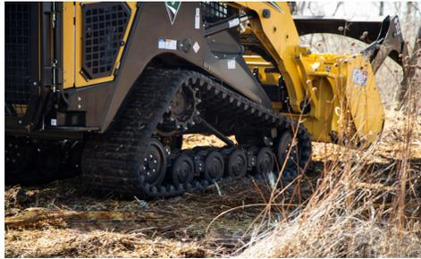
**TRACK SUSPENSION.** A torsion suspended track system provides a comfortable, swift, durable and tractive drive system for the most demanding terrain.
