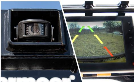
**REARVIEW CAMERA WITH IN-CAB MONITOR.** An in-cab monitor provides added visibility, enhancing maneuverability.
