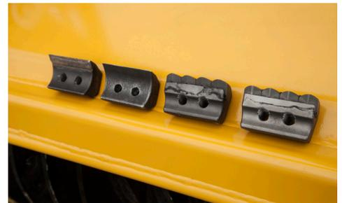
**ABOVE-GROUND MULCHER – INTERCHANGEABLE ROTOR TIPS.** The interchangeable rotor tips allow the operator to optimize cutting performance to fit site conditions, without the need to rebalance the drum each time.
