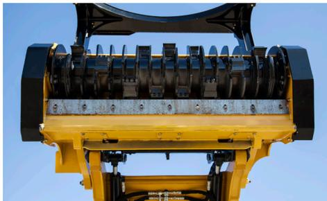
**ABOVE-GROUND MULCHER – RINGED ROTOR.** The ringed rotor design of the above ground mulcher head attachment helps guide material into the path of the cutting tips for effective single-pass clearing and full-tip coverage. By controlling the depth of cut, the engine can be loaded to peak operating performance.
