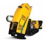
SERVICEABILITY. The drill's flip-up metal hood offers ease of access when performing routine service and maintenance.
