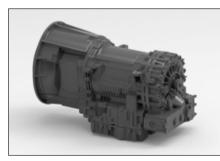
Planetary powershift transmission optimizes shift points to match conditions and vehicle weight while protecting the transmission from operator error and abuse.
