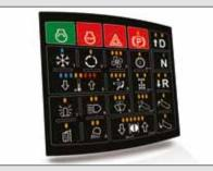
Convenient sealed switch module provides fingertip control of numerous productivity enhancing functions including: **Keyless Start, I-Tip, Dump Body Upper Limit, Soft Stop/Hard Stop Selection, Retarder Aggressiveness and Speed Control.**
