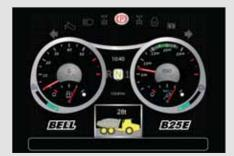
The exclusive on-board weighing option presents the operator with real time information on the payload while the machine is being loaded. A 'speed restriction' mode can also be activated if the machine is significantly overloaded.
