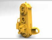
The transfer case inter-axle differential delivers equal torque to each axle when traction is favorable. When conditions deteriorate, the diff-lock automatically engages to deliver torque to the tires that can best use it.
