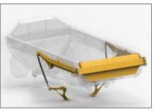
A tailgate is available as an option for better material retention. The tailgate opens as the bin is raised for dumping. Spring steel straps maintain positive seal throughout the haul, ensuring minimal material is lost.
