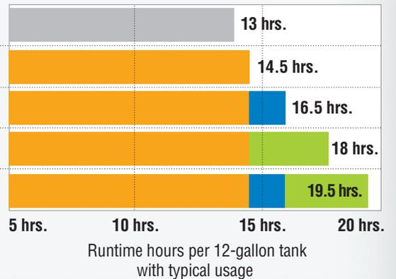
\*Based on typical usage — 150 amps welding 40% of the time; 20 amps generator power 30% of the time; and idling without load 30% of the time.
