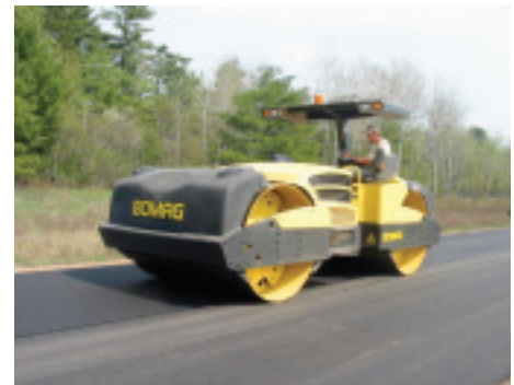
84" rolling width with available 4000 vpm frequency.
