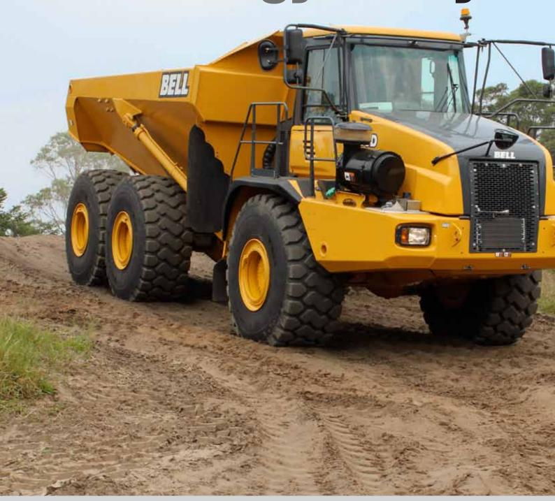
Bell Equipment has implemented on SCR system to meet stage 3b emissions standards. Called Bell Blu@dvantage™, it is an SCR package designed specially for the off-highway market.
