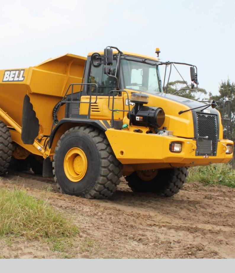
Add enhancements such as a Stage 3b emission-certified engine, solid state electrical system and spacious, redesigned cab with refined controls, and you have everything you need to maximise uptime and productivity.
