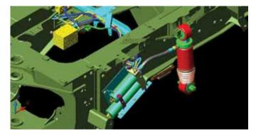
The front suspension consists of independent suspension cylinders that allow the oil flow and pressure to be constantly changed to minimise the effects of machine movement. Sensors in the frame continually measure and accommodate for bumps in the surface while lateral sensors also measure any roll and constantly adjust cylinders to accommodate for this.
