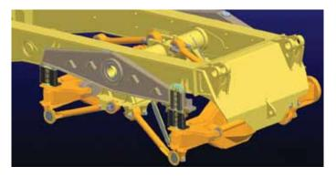
The incorporation of the dual stage sandwich block allows for differing suspension characteristics between laden and unladen runs. The simple mechanical solution has proved durable while being extremely effective in smoothing out the ride.
