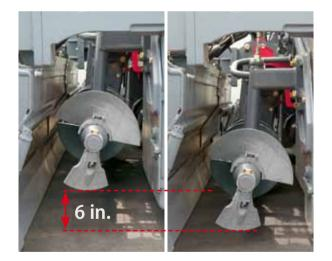
Hydraulically adjustable augers are infinitely variable in height within a range of 6 inches. Hydraulic auger height adjustment (including bearing boxes and limiting plates for the auger tunnel) provides optimal spreading of the material even when paving thin layers or on sections where thickness varies.
