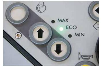
Three engine speed ranges are available which are selected conveniently at the push of a button (MIN, ECO, MAX).
