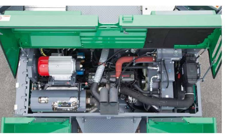
The VISION 5200-2i paver reaches laydown rates up to 1,300 tons of mix per hour. For this high performance, a powerful engine is installed. With an output of 250 h.p. at 2,000 rpm, the Cummins engine is a real powerhouse. It complies with the current exhaust emissions standards Tier 4i.
