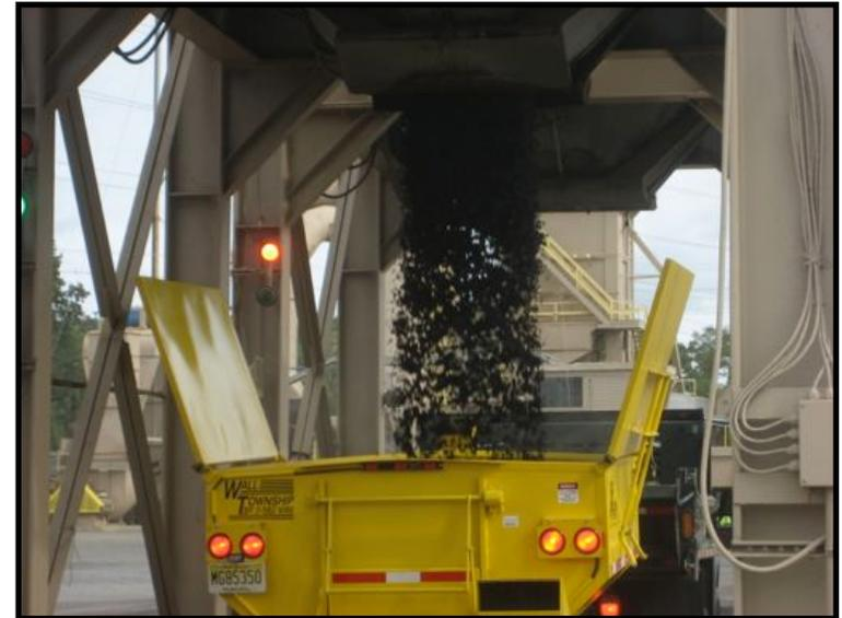
**3-Ton Trailer Loading at the Asphalt Plant**
