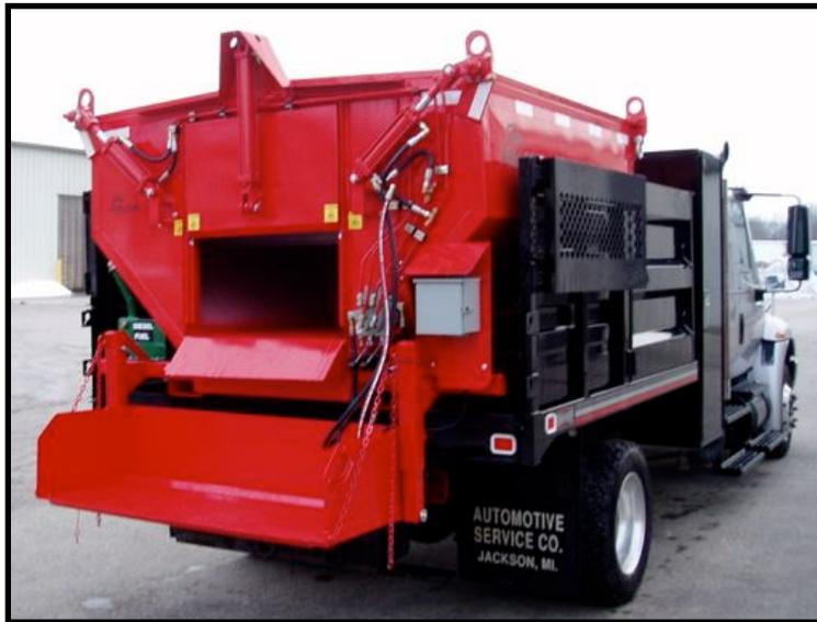
**6-Ton Slip-in Mounted on Dump Truck**
