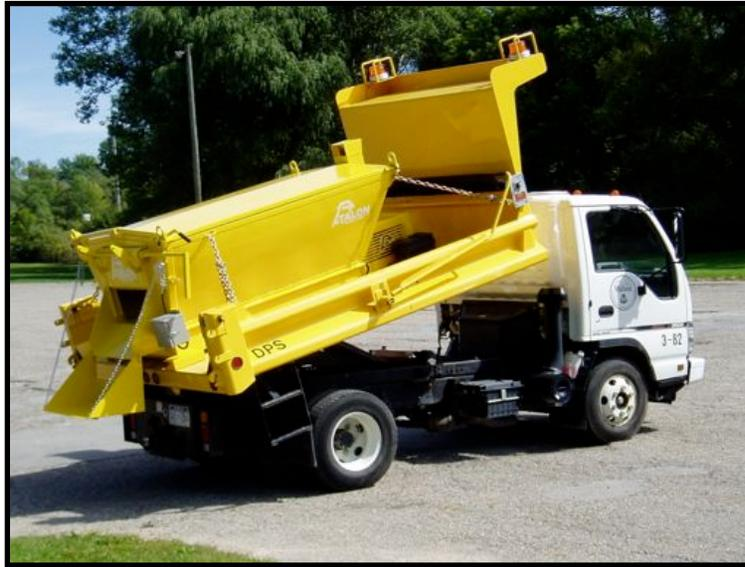
**2-Ton Slip-in Mounted on Dump Bed**
