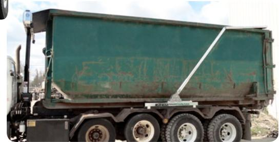
bumpers on bow contact the rear of the container. After the adjustable tower is lowered, the tarp can be 'winched' onto the container to provide a snug overall fit.
